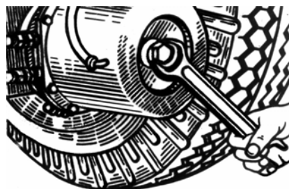
Figure 9 – Unscrewing the pusher accumulator fixing bolt
