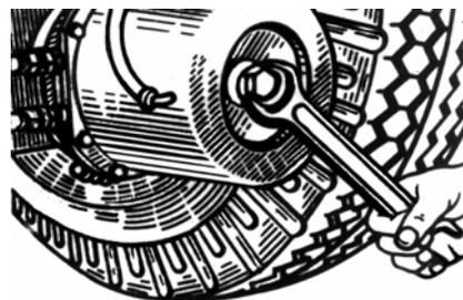
Figure 8 – Unscrewing the pusher accumulator fixing bolt
