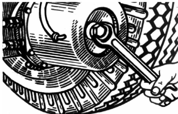
Figure 12 – Unscrewing the pusher accumulator fixing bolt
